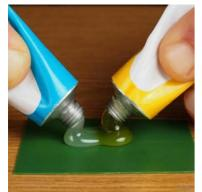
Epoxy Resin comes typically as two resins that need to be mixed together before use.
