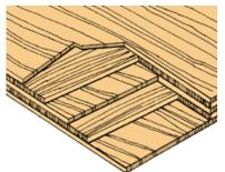
Layers of hardwood veneer are bonded together with the grain direction in each layer laid at 90 degrees to the previous layer.
