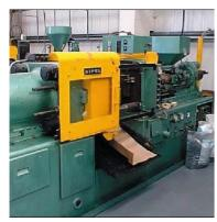
HIPS, and other member of the styrene family, is widely processed through all the standard techniques—such as injection moulding.
