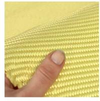
Kevlar fibres are woven into a cloth that can absorb force that would cause serious injury.
