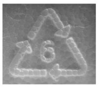
Expanded Polystyrene can be recycled and is represented by a number 6 in the recycling symbol.
