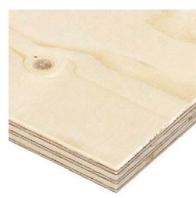
Plywood uses laminated veneers to produce large sheets of stable material with a natural wood finish.
