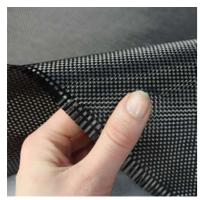
Carbon Fibre consists of shiny black fibres drawn from approximately 90% carbon.
