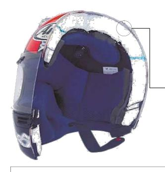
Inside the outer shell of a crash helmet is the impact absorbing liner, usually made of expanded polystyrene. The function of this layer is to absorb impact. The polystyrene compresses absorbing much of the impact. This system is designed to work one time. That's why a motorcycle helmet should be thrown away after being involved in a significant blow.
