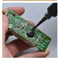
Epoxy Resin is a good electrical insulator.
