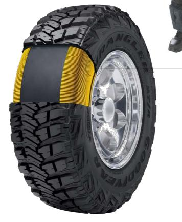
Kevlar fibres offer superb puncture, abrasion and tear resistance. Other benefits include a quieter ride and a reduction in rotational weight, which can help decrease engine strain, and typically results in improved fuel efficiency.
