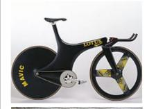
Carbon Fibre's high strength to weight ratio make it a good material where weight reduction is important for performance
