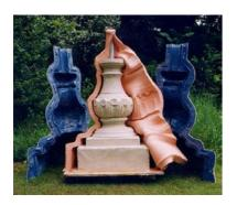
A mould is required for production in GRP.
