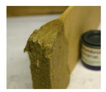
MDF can be easily damaged by moisture.
