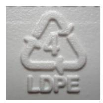
LDPE can be recycled and is represented by a number 4 in the recycling symbol.
