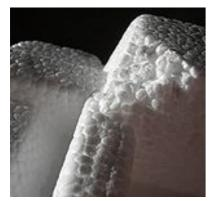
It is usually white in colour and made of pre-expanded polystyrene beads.
