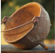
Cast Iron can have poor corrosion resistance.
