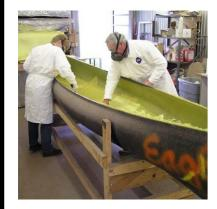
Laying up is the term used for the process involved in manufacturing with GRP.
